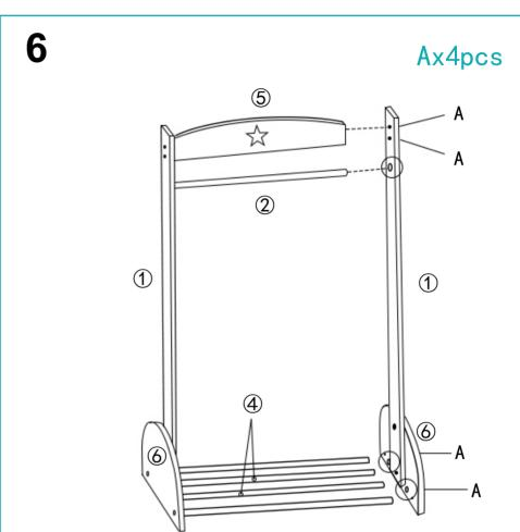
Step 6:Use Part A to install the other side with the frame.
