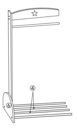
Step 4: Install 4 into 6 without screws.
