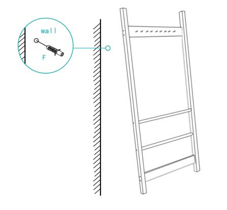
Step 4: Install Part F into the wall.
