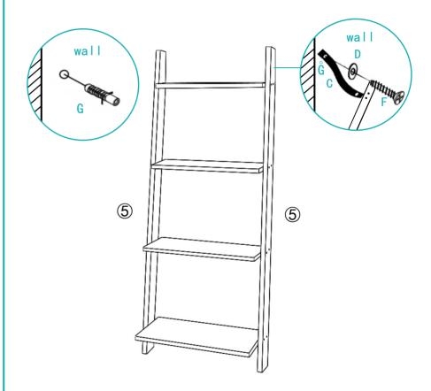
Step 4:First install Part G into the wall. Then use Part D and F to connect with Part G.
