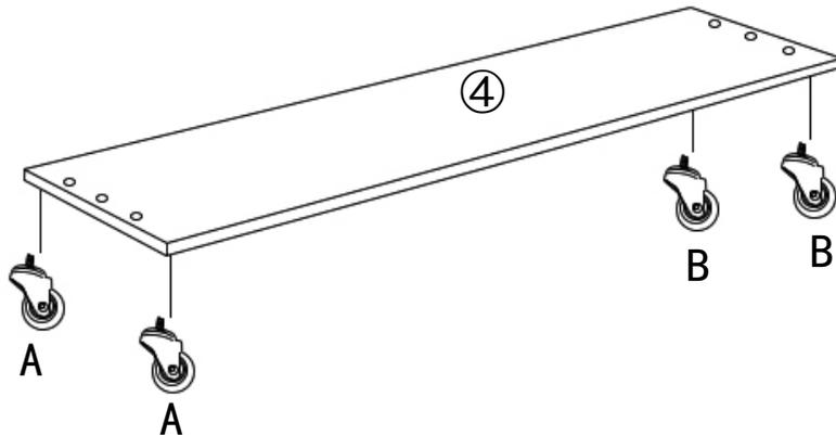
Step 3: Use Part E to connect Part A, B and ④.
