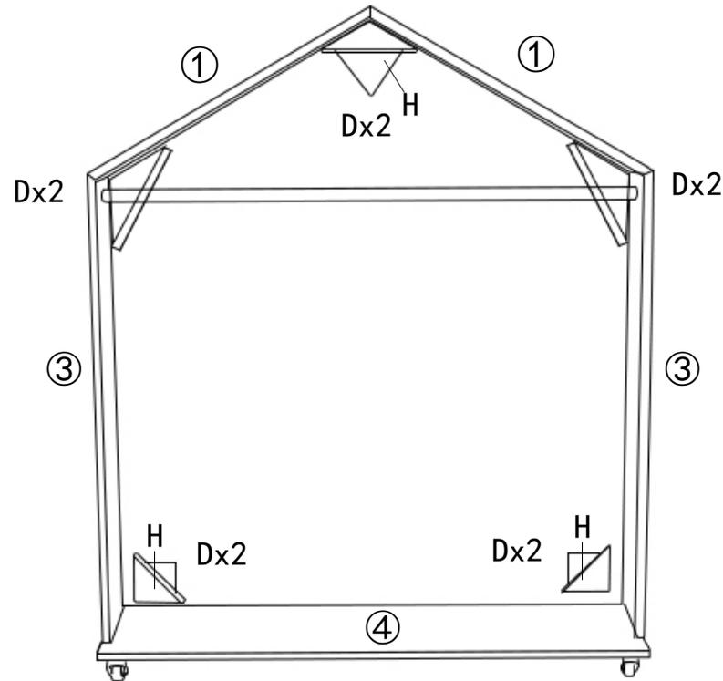
Step 5: Use Part D to connect Part H with ①, ③ and ④.
