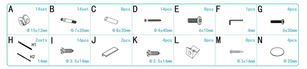
$\Phi:$  it means the diameter of the product; e.g.  $\Phi\,6$  means 6mm diameter.
